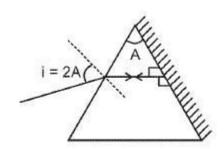
Applying Snell's rule between the incident ray and the refracted ray, we
